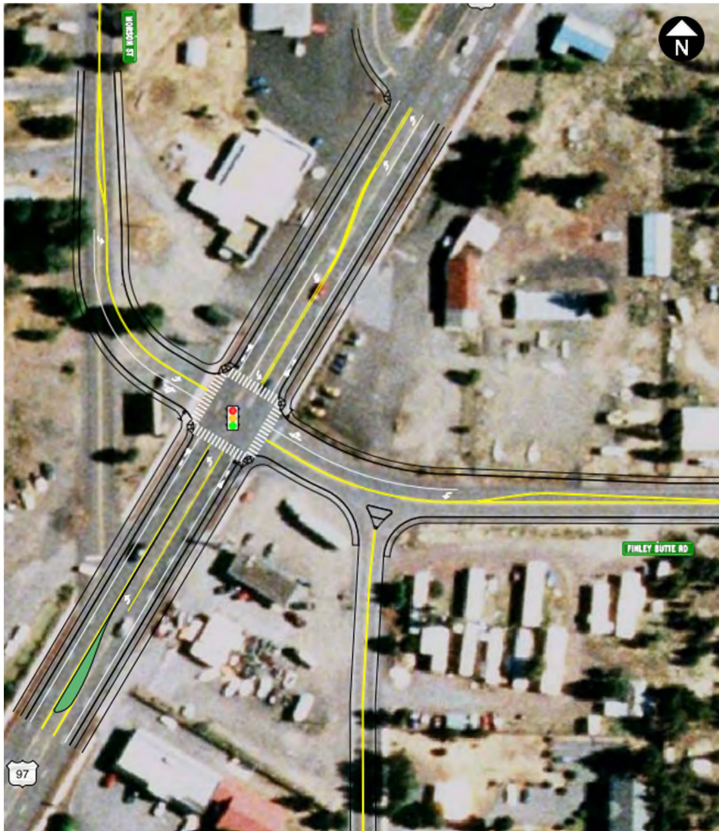
Figure 4. Conceptual US 97/Finley Butte Road – Morson Street Improvement. Source: US 97/La Pine Corridor Plan.
