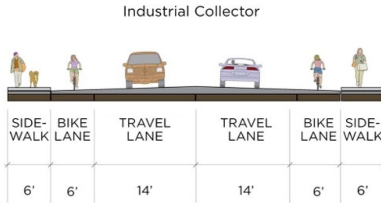
Figure 3: Industrial Collector ROW standards from TSP
